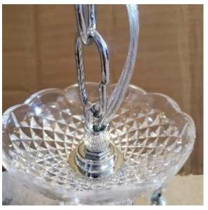
c) Gather chain and power cord in one hand and rotate connector counter clockwise approximately 6 turns. While maintaining tension in cord and chain, seat connector onto exposed threaded rod and screw clockwise until the connector is fully engaged
