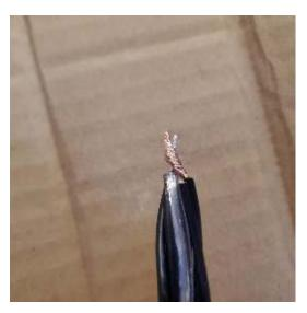
d) At this step you have 2 groups of black wires, 2 groups of white wires, and your separated power cord ends. You now need to take both groups of matching coloured wires and one power cord wire end and twist them together like you did with the wires in previous steps. Do this for both the black and white wires. Remember to always twist in a clockwise direction.
