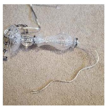
a) In this step you will need the assembly from step 1, shown in the picture on the left. You are going to feed your power cord through this assembly, starting at the top where the crystal cup is(the left side in the photo)
