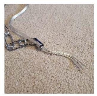
For this step you will need the power cord, and chain. Feed the cord through the connector at the end of the chain until you have about 2 feet of cord exposed through the chain. (See photo below)
