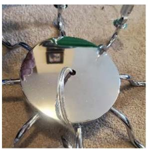
a) Once you have confirmed your power is working, you need to place the hub cap(that you threaded the power cord through earlier) on top of the dish that contains all your wiring. Be careful to ensure no wires are pinched between the hub center and cap.
